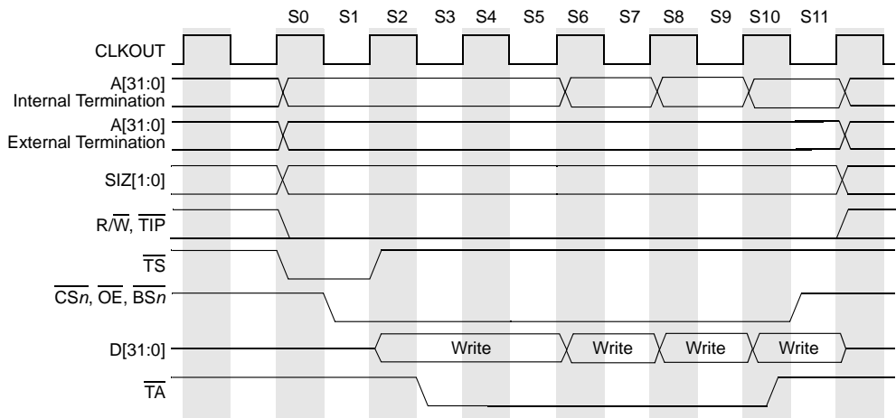
Figure 13-16. Line Write Burst (2-1-1-1), Internal/External Termination
